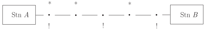
Fig. 6. Guideway: stations A and B are connected by a single one-way track from A to B. The track consists of 4 sections, with stoplights (*) and detectors (!) installed at various section junctions as displayed.
