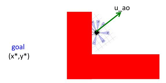
If too close to an obstacle (unsafe), use AvoidObstacle control.
