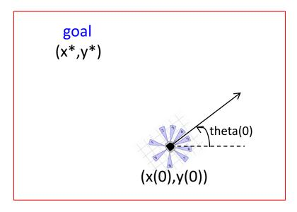
Assume robot is moving at <u>linear velocity v=constant</u>.
